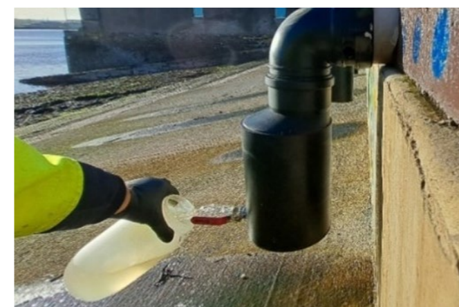
Cork County Council environmental technicians are undertaking a 12-month monitoring regime of the raingardens. Samples of rainwater run-off from the adjacent street are tested for contaminants to assess the most suitable system for future raingardens in Cobh.
