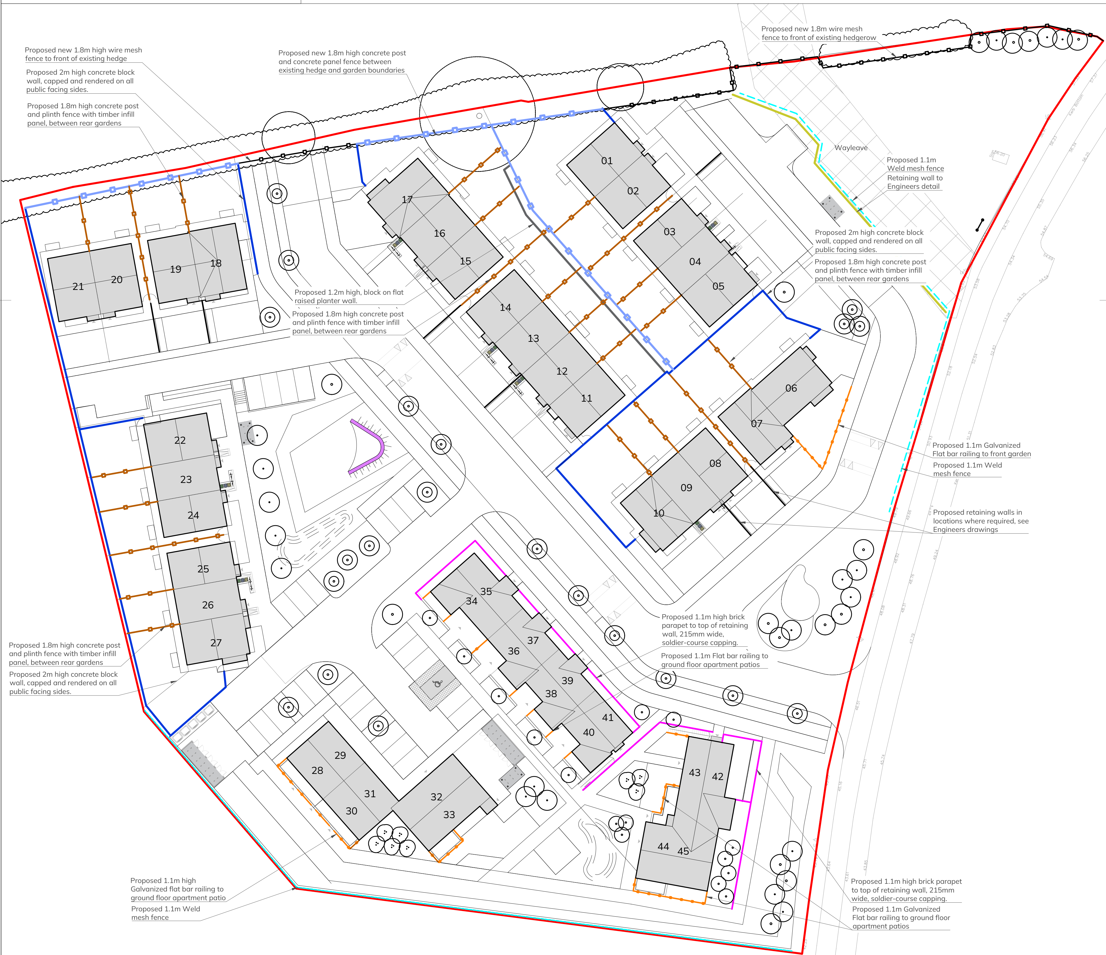
Boundary 5 - 1.8m high wire mesh fence Scale 1:50 @A1
